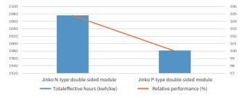
Figure 4-1 Comparison of power generation performance between Jinko N-type double-sided module and Jinko P-type double-sided module
